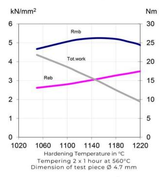
Rmb = Ultimate bend strength in kN/mm<sup>2</sup> Reb = Bend yield strength in kN/mm²
