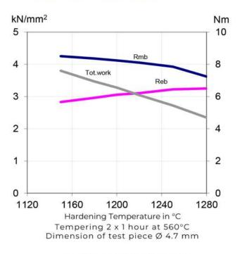
Rmb = Ultimate bend strength in kN/mm² Reb = Bend yield strength in kN/mm² Tot. work = Total work in Nm
